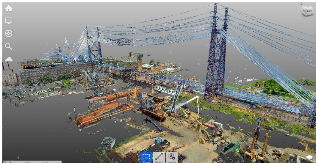
Figure 1 – 3D scanning generates point cloud data
